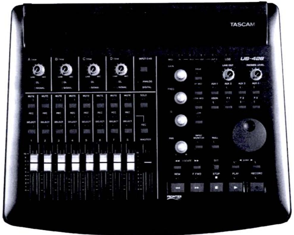
The US-428 attaches to the computer via a single USB cable. You don't ever have to open up the computer. Heck, you don't even have to reach around the back—just plug it into one of the front-panel USB jacks!
