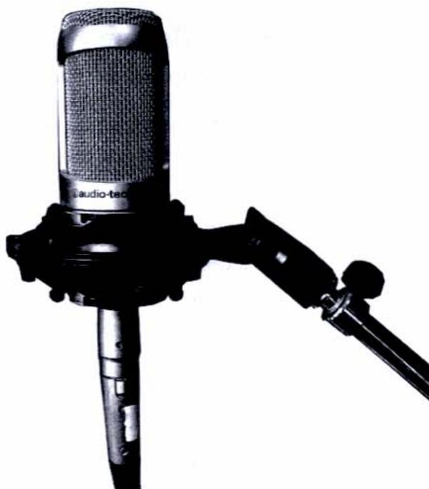
Unless it runs on batteries, a condenser mic requires *phantom power*, a 48-volt signal that reaches the mic via the three-conductor microphone cable. Although it has mic inputs, the US-428 doesn't offer phantom power, so I'll have to add a small phantom power supply between the mic and the XLR input on the US-428. I've chosen Stewart PM-1, which costs about \$80 (see Figure 4-8). It may be an extra step, but it's worth taking for the quality that a condenser mic affords.
