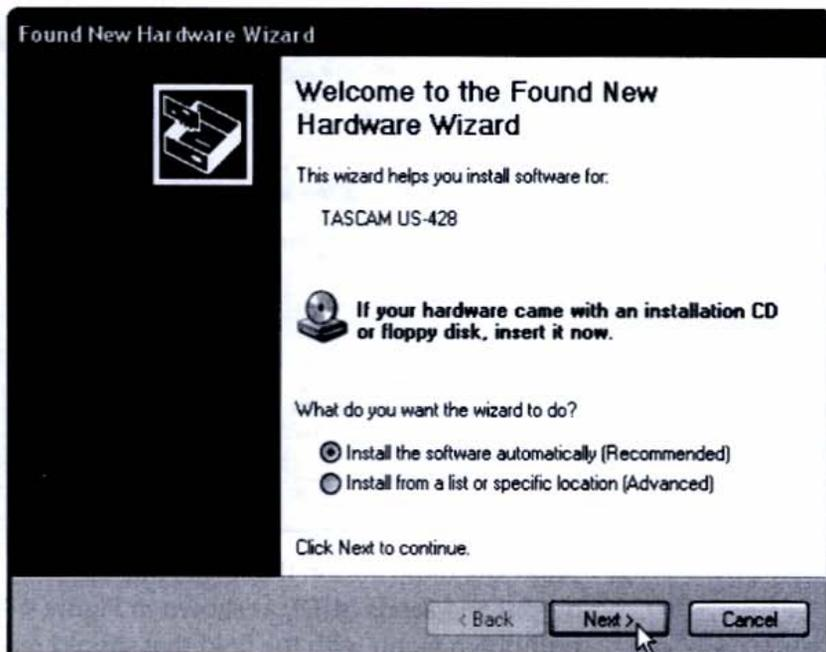
After you follow the steps for installing the necessary software and drivers, your interface will be ready for operation. If the hardware wizard reports an error in the setup process, repeat the steps and read the prompts carefully. It's possible you may need to get an updated driver from the manufacturer's Web site.
