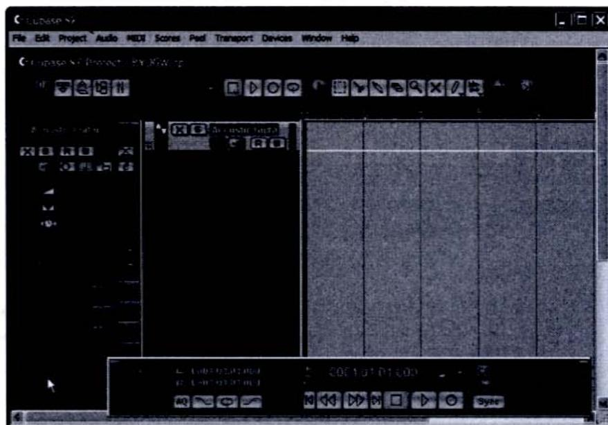
In the Inspector, set the Acoustic Guitar track to receive Input 1. Plug your microphone into the US-428's Channel A, turn on your phantom power supply, and start singing, playing your acoustic guitar, or making some other kind of noise. You should hear yourself through the US-428's audio outputs (speakers or headphones).
